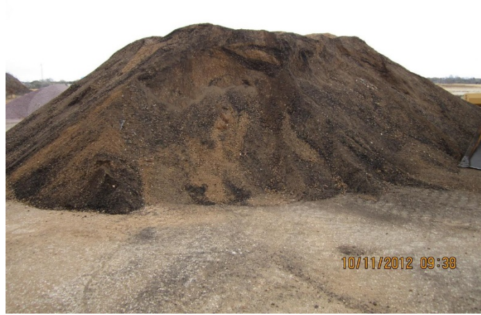
Figure 9 Shingles and Gravel Stockpile (Thomas J. Wood et al. 2014)
