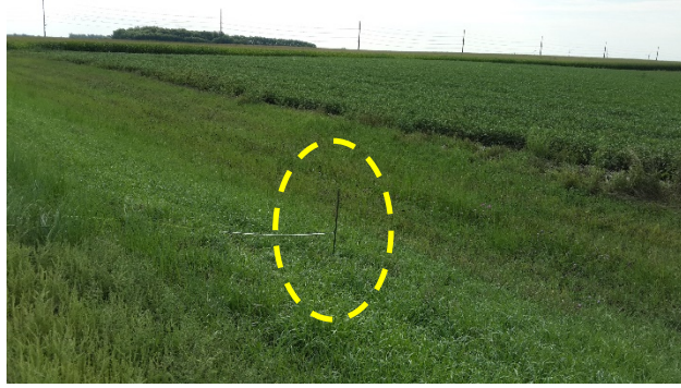
Figure 18 End Indicator-Steel Pin (Photo by the Author)
